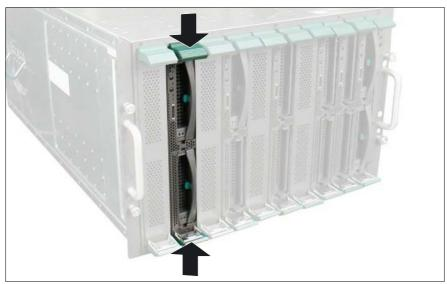
Figure 33: Final engaging of the locking mechanism
